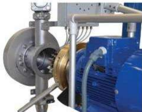
Improper die sizing can cause a variety of pellet-quality problems in underwater pelletizing. Pictured here is Gala's Model 7 EAC Pelletizer showing the cutter hub and the cutting chamber, with a bit of the downstream side of the die visible.
