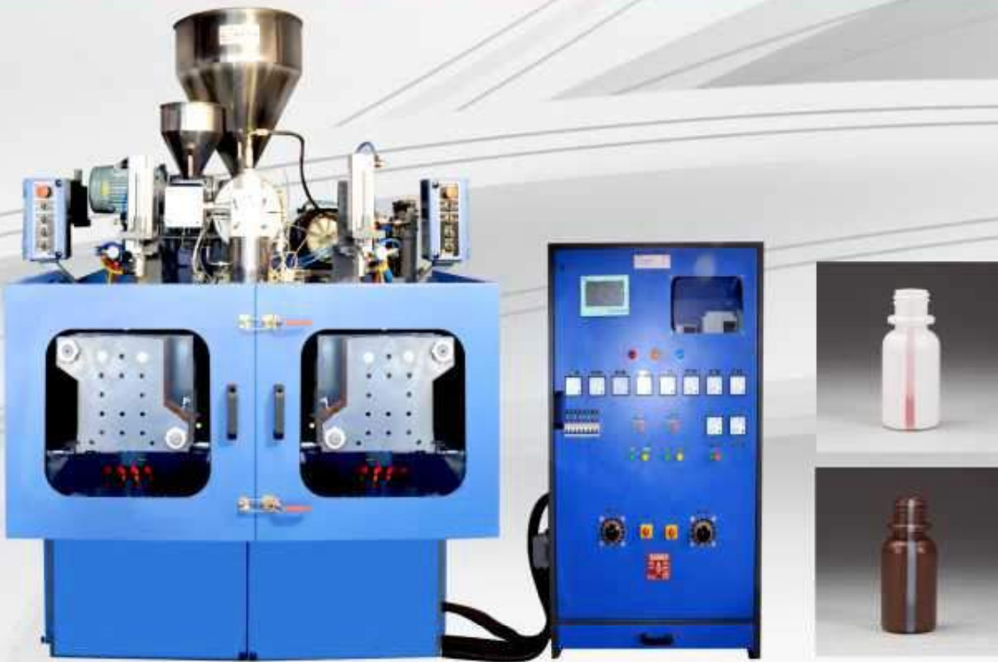
1000 ML Double Station V- Strip Plastic Extrusion Blow Moulding Machine
