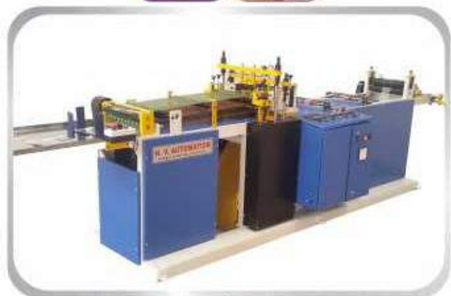
Automatic Cut & Seal For "U" Shape PVC Pouch only 3mm Waste
