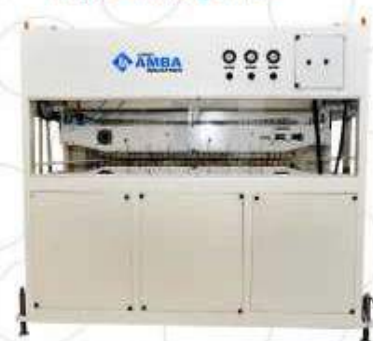
Tube Pipe Traction Unit
