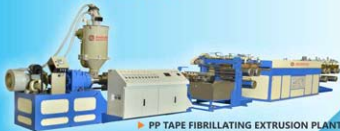
▶ PP TAPE FIBRILLATING EXTRUSION PLANT Production Capacity 100 to 235 kgs/Hrs.
