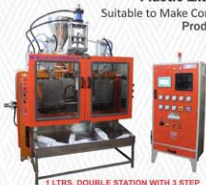
1 LTRS. DOUBLE STATION WITH 3 STEP PARISON CONTROLLER
